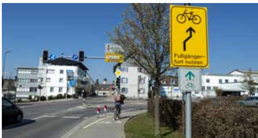
■ Thanks to clear bicycle path guidance measures, it is now much harder for cyclists to ride straight on dangerously without using the pedestrian crossing.
