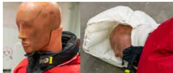
■ Airbag helmet in "normal" and inflated state.
